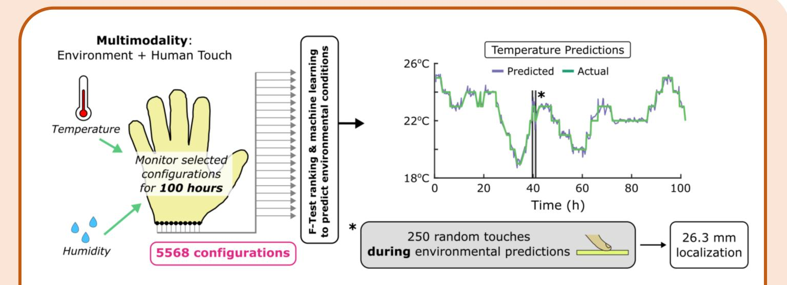
The hand's hollow skin can simultaneously predict environmental conditions, generate proprioceptive signals, and localize human touches to 26 mm over the front and
