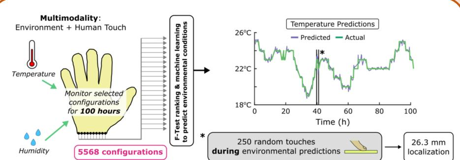
The hand's hollow skin can simultaneously predict environmental conditions, generate proprioceptive signals, and localize human touches to 26 mm over the front and back of its 380 cm<sup>2</sup> area.
