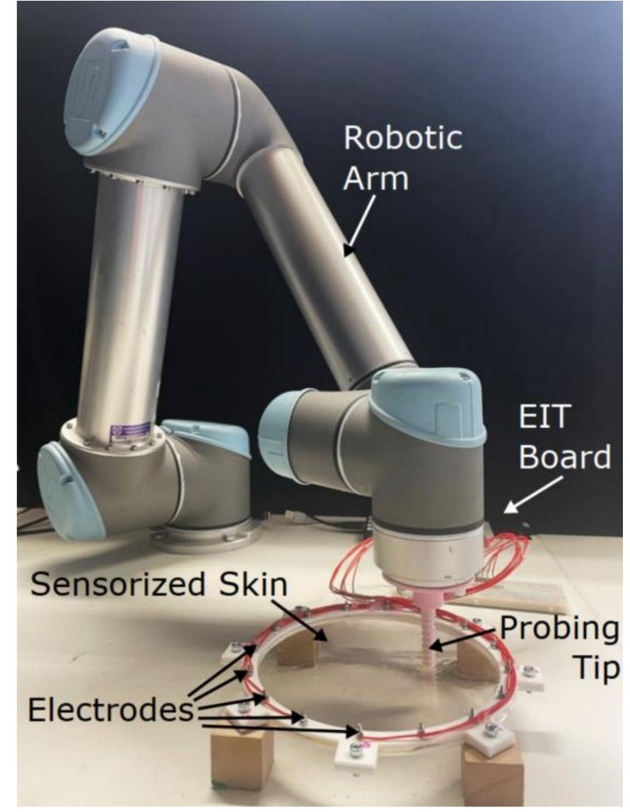
• Electrical Impedance Tomography (EIT) attaches multiple electrodes to the material's perimeter, using the properties of the skin itself as the body's sensory layer.
